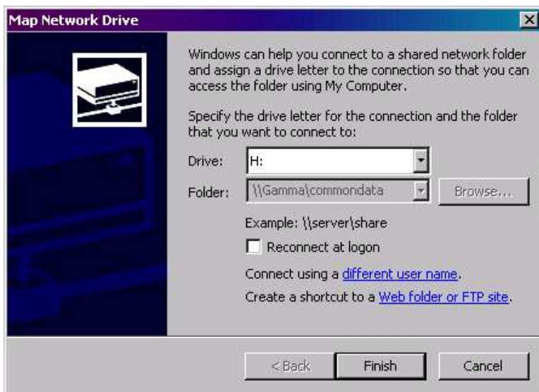
Figure 19. Mapping a drive letter to a share on another Windows computer via the Map Network Drive called from a share's context menu in Windows Explorer.
