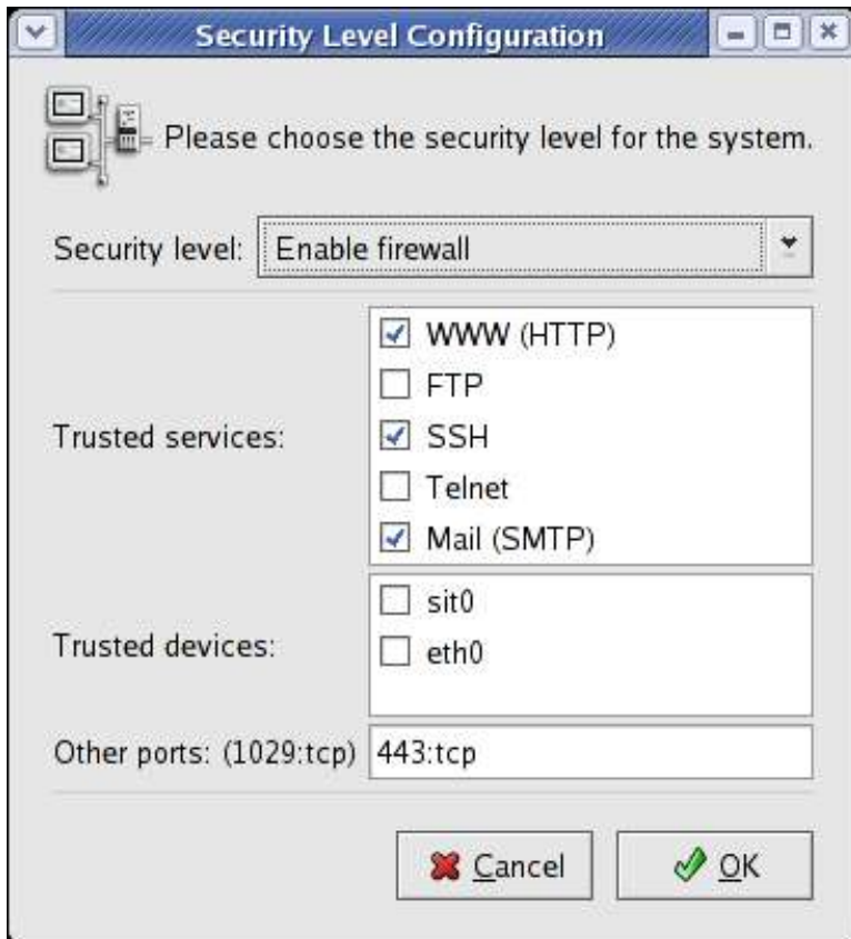
Figure 4. The appropriate settings for setting up a firewall on your Web server.
